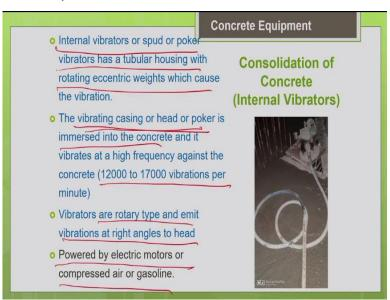
So, first let us discuss about the internal vibrators which are very commonly used for the consolidation of the concrete. We call them as needle vibrator or spud vibrator or the poker vibrator. So, there are different names to call these internal vibrators. These are more effective forms of vibrators, because what we do is basically this needle vibrator has a casing or the head at the bottom.
