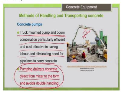
So, in some places the job site will be very much congested that it will not be possible to place the pipelines on the ground. So, in that case, you can go for this truck mounted pump and boom.
