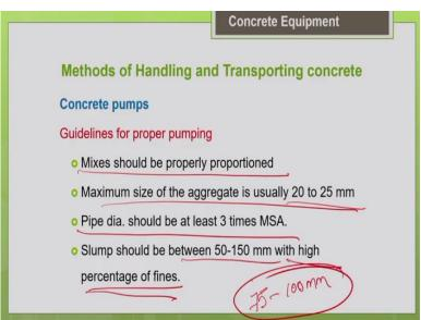
So, there are some guidelines for proper pumping or successful pumping. That we should always keep in mind. So, basically if you decide that you are going to go for pumping method for the concrete placement that decision has to be made even during the mix design itself. So,
