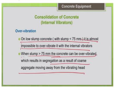
And another thing you should keep in mind is we should never over vibrate the concrete. So, if you over vibrate also the it will result in segregation of your concrete. So, generally the chances for over vibration will be there only in highly consistent mix in flowable concrete. So, when you handle the stiff mixes the chances for over vibration is very less. On a low slump concrete with slump less than 75 mm, it is almost impossible to over vibrate with internal vibrators.
