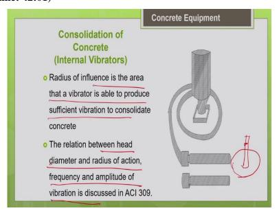
So, basically every needle vibrator, it will have its own radius of action. So, this is the casing or the head you can see. As I told you at the bottom, you have the casing or the head. So, how much will be the area of influence? So, this is your head, how much will be the area of influence? So, that depends upon the diameter or the radius of your the head. So, this this casing head this diameter will determine the radius of the influence.
