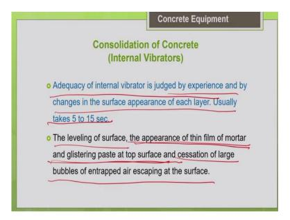
So, how long I should vibrate do the vibration at a particular place. Usually we take approximately 5 to 15 seconds. But it depends upon the consistency of the concrete. Generally, based upon experience what the worker will do is by looking at the concrete itself by looking at the concrete surface itself he can make a guess whether the consolidation is done or not. If he is an experienced person, he can make a guess whether the consolidation is done or not.
