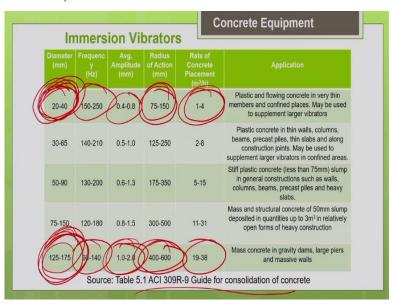
So, you can get this information in ACI 309R which gives you the guide for the consolidation of concrete. So, you can see this table is taken from the ACI 309R. The basically you can see there are different types of vibrators available with diameter ranging from 20 mm to 175 mm. You can see. So, there are lot of options available. So, depending upon the thickness of your section and depending upon your placement rate needed accordingly you can go for the particular diameter of your vibrator.
