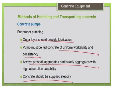
So, what are the other guidelines? Let us see. So, as I told you, the important thing is before pumping of your actual batch of concrete, you have to do some lubrication. So, that lubrication will only facilitate easy flow of your concrete through the pipeline. And we should feed the
