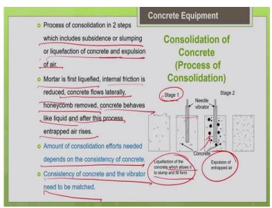
So, basically before moving into the types of vibrators, let us discuss about the actual process of consolidation. How this process of consolidation is happening in the concrete? So, the consolidation usually occurs in 2 steps. The first thing is when you put your vibrator in the concrete, so, what is happening is your concrete becomes liquefied. It will behave like a liquid. It will start flowing laterally.
