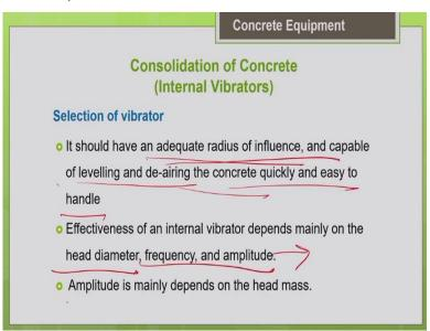
So, whatever vibrator you choose, it should have a adequate radius of influence so that you can have your desired consolidation rate. You can see your rate of concrete placement also varies. For a smaller vibrator, you can see 1 to 4 meter cube per hour. But for a bigger diameter vibrator you can have 19 to 38 meter cube per hour the concrete placement. So, depending upon the productivity needed, so, you have to make the choice of your vibrator.
